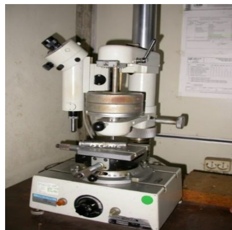
Gambar 6. Alat Uji Kekerasan (Vickers) HV Frank Finotest
