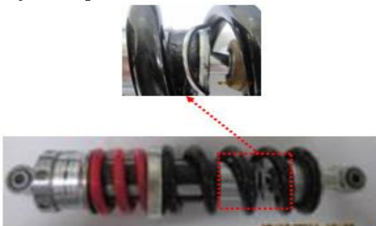
Gambar 3. Crack Area Rolling Damper
