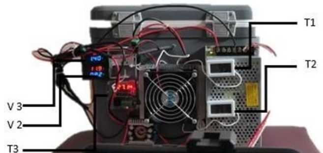
Gambar 2. Sistem pendingin cooler box
