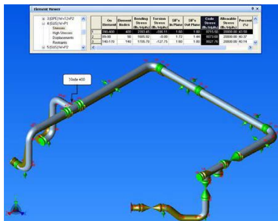
Gambar 4.1. Permodelan tegangan pipa akibat Beban Sustain (Sumber : Program CAESAR II)
