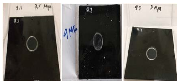
Gambar 4.9 Hasil pull of test suhu pengovenan 220°C
