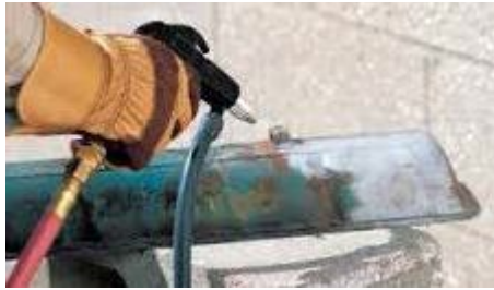
Gambar 3.3 Proses sand blasting
