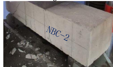
Fig. 9 Crack pattern of NBC-2
