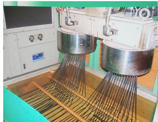
Fig. 3c Fibre Drawing Process
