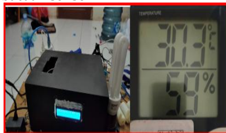
Gambar 12. Perbandingan Sensor DHT11
