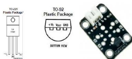
Gambar 2.2 Sensor suhu LM 35
